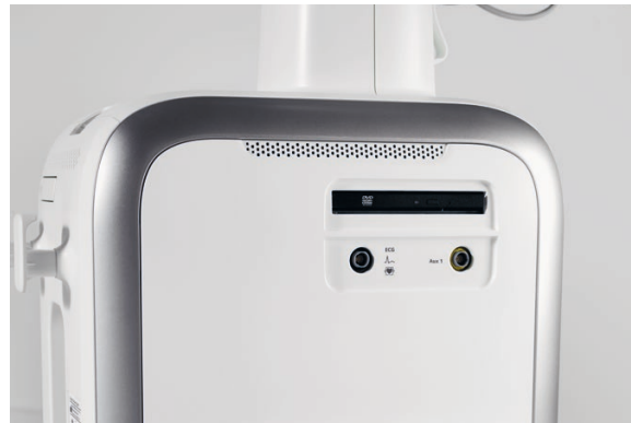
ECG cable connector, auxiliary physio port, and DVD writer.
